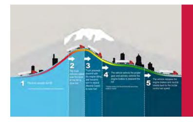
Predictive Cruise Control employs GPS and digital terrain mapping technology to anticipate changes in grade over a mile ahead. Using these inputs, the technology automatically modifies the cruise control set speed in order to maximize fuel economy. Up to 3% fuel savings in possible when the vehicle is driven on rolling hills and coupled with neutral coast.
